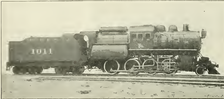
D. & H. 2-8-0. WITH CENTRALLY PLACED CAB. SAME DESIGN AS NO. 1054.
